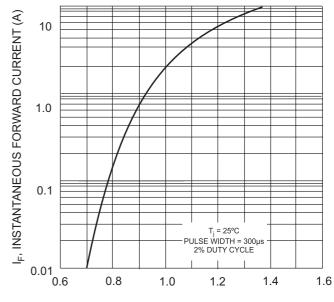
V<sub>F</sub>, INSTANTANEOUS FORWARD VOLTAGE (V) Fig. 2 Typical Forward Characteristics
